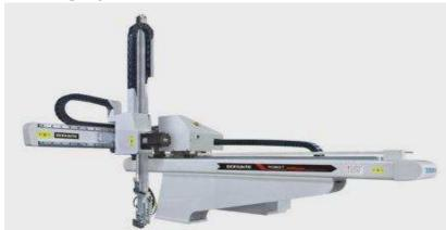
BRB800 Series is applicable to all types of horizontal injection machine ranges of 100~250T for take-out products and sprues. Vertical arm is single stage, suitable for two plate mold products take out. Traverse axis and vertical axis driven by AC servo motor. After installed this robot, the productivity will be increased 10~30%, reduce defective rate, ensure safety of operators, reduce manpower and accurately control the output to reduce waste.
